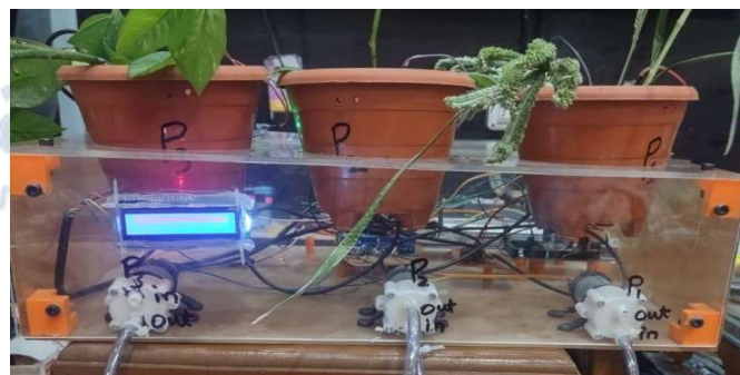
Fig 4: Water Requirement Prediction System Front View
