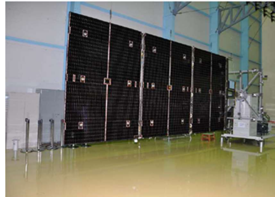
Fig 9: A typical multi panel solar array
