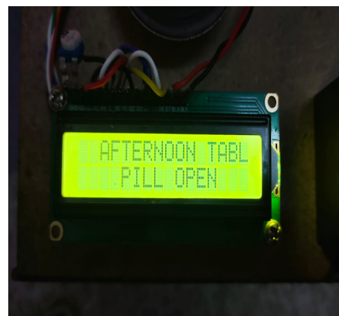
Fig 7 :Display of pill box open on LCD
