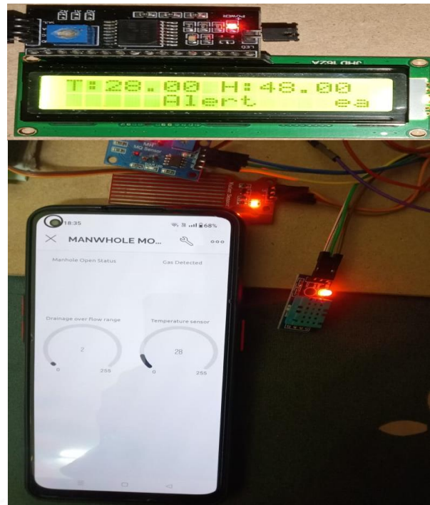
Fig 4: Testing of temperature sensor and output is displayed in Blynk app, LCD
