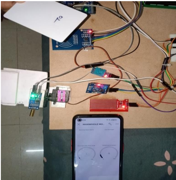
Fig 6: When RFID card is again scanned, manhole cover is automatically closed and output is displayed in Blynk app
