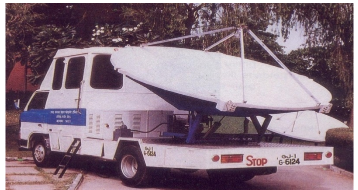
Fig 14 Transportable Communication Terminal
