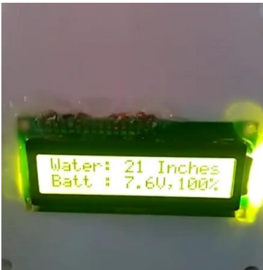
Fig7.2: model shows the Water level at 21 Inches and battery percentage
