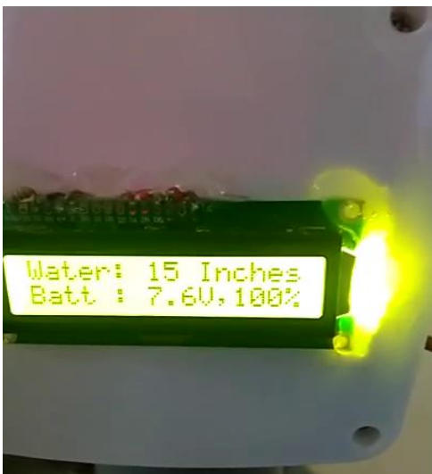
Fig 7.4: model shows the Water level at 15 Inches
