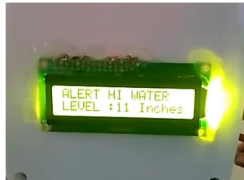
Fig7.6: model shows the Water level at 11 Inches
